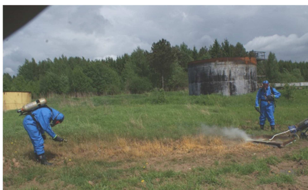
Figure 1. Full-scale tests: a) measurements of the concentration near the emission source, b) height profile of chlorine concentration \approx 100 m away from the source [5].
